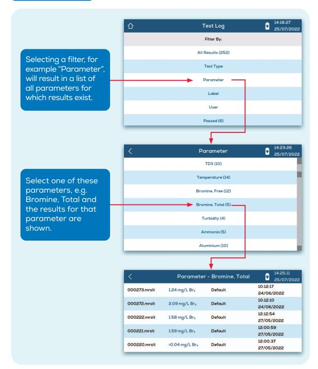
If limits are set for a parameter the results are colour coded to indicate if the result is within the pass and fail limits set.
