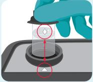
Align tubes as shown. Always use the tube cap as it excludes light from the optics.
