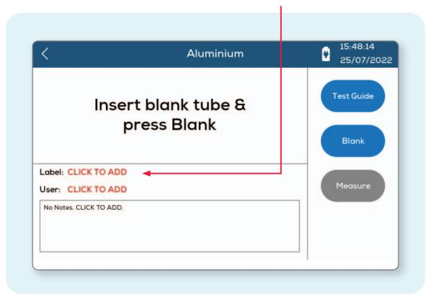
Lumiso can be set to prompt the user to attach a label to each result. (See: Setting Pass and Fail Limits for a Test).
