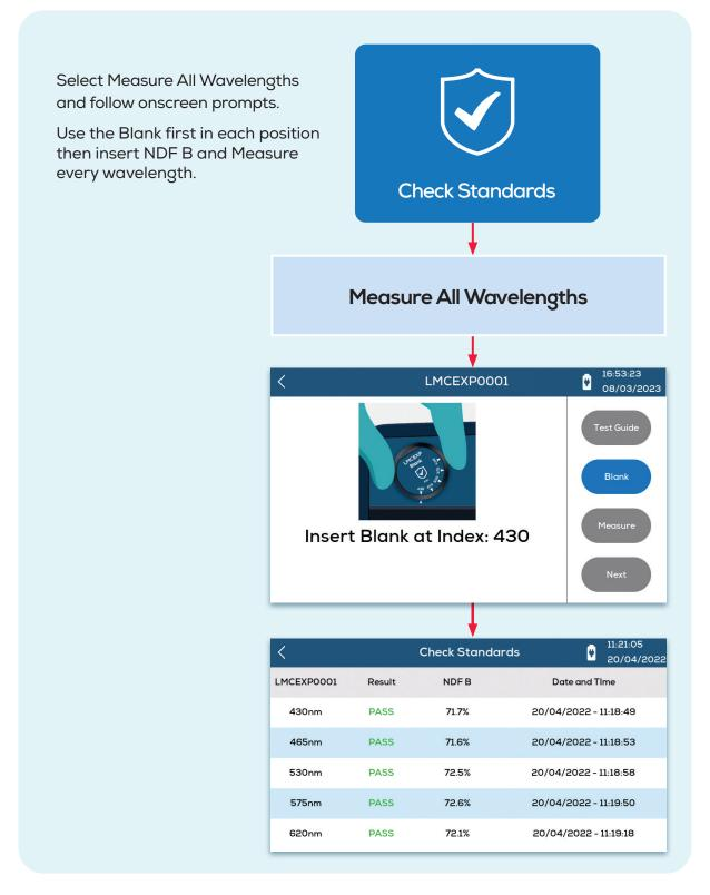
**Note:** There is also an option for checking a single wavelength.
