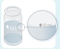
Measure volumes accurately as shown (or use a pipettor or syringe).
