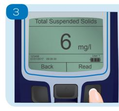
An audible tone will sound at the start and end of measurement. Result is displayed on the screen in mg/I and stored in the log with time, date, Operator ID and Sample ID.
