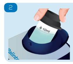
Insert the tube with the orientation mark ◊ facing forward and press read. An audible tone will sound after each reading.
