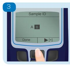
To delete characters press and hold the [Del] key. Select 'Done' to save the ID. Up to 24 Sample IDs can be created.
