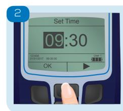
Use up/down keys to adjust the hour; press the right key to select and adjust the minutes. The time is displayed in 24Hr format.
