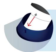
Place the sample tube in the instrument in the same orientation for all readings .
