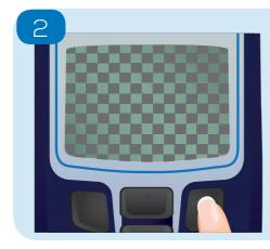
The LCD screen contrast can be manually adjusted. Use the up/down buttons to adjust the contrast until the alternating shapes are clearly visible and press 'Save'.
