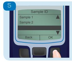
To record results without a Sample ID. Select a blank entry by scrolling to the bottom of the list and select 'Back'.
