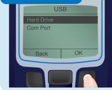
To download results and calibration logs, or to update the instrument firmware the device must be in 'Hard Drive' mode .
