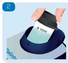
Select the Sample ID for the site/sample. The calibration data will be recalled automatically. Insert the sample with the orientation mark § facing forward and press 'Read'.
