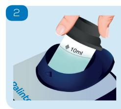
Insert the sample with the orientation mark ◊ facing forward and press 'Read'. An audible tone will sound at the start and end of measurement.
