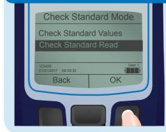
Select the Check Standard Read option to perform a recorded read back of each turbidity check standard.
