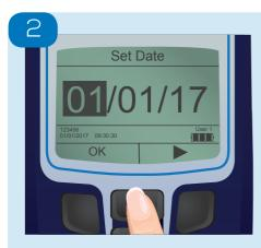
Use the up/down keys to adjust each value in the date display, using the left/right keys to select the field. The date format can be set to either DD/MM/ YY or MM/DD/YY
