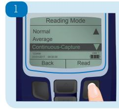
This mode performs repeated Normal readings of the sample until stopped by the user.
