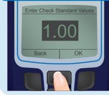
Use the up/down keys to adjust the displayed values to match the assigned target for each check standard. 23
