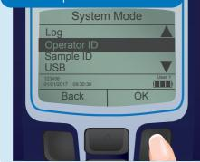
To access operator ID from the home screen press 'System' mode then 'Operator ID'. Up to 12 Operator IDs can be created. When selected, the ID will appear in the info panel on screen as well as in the log.
