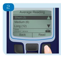
Select the number of readings required: Short (3), Medium (6), Long (12). Insert the sample with the orientation mark ◊ facing forward and press 'Read'.
