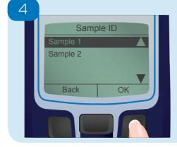
Select 'OK' on the Sample ID to be used. When selected, the ID will appear in the information panel on screen as well as in the log when results are stored.
