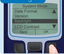
The instrument display features a high intensity backlight for use in low light conditions. Select either 'On' or 'Off'.
