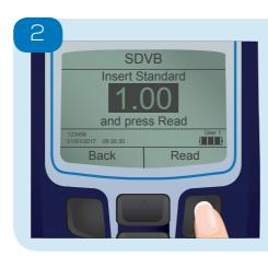
Use the Up/Down buttons to adjust the value on screen to that on the standard and press 'Read'.
