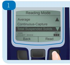
This mode will only be active if a site calibration has been stored within the Turbimeter. Once a calibration has been created, the Sample ID can be used to recall the site specific relationship between turbidity and suspended solids.
