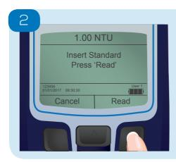
Follow the on-screen prompts and insert the Check Standards as requested. Select the Read button to perform the measurement.
