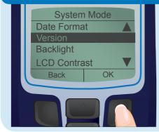
From the main menu select 'Sytem mode' then 'Version'. The serial number of the instrument and the software version are displayed.
