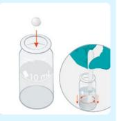
Prepare sample by adding an Alkaphot tablet. Thoroughly crush and stir, until fully dissolved.
