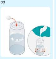
Prepare sample by adding an Aluminium No1 tablet and crush and stir.
