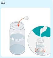
Then, add an Aluminium No2 tablet. Vigorously crush and stir.
