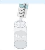
To a clean photometer tube, add a fresh 10 mL of sample.
