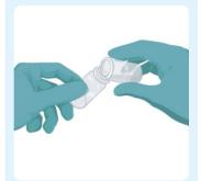
Pour a few drops of this treated sample into another clean tube. Keep the remainder. 10
