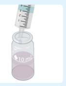
Fill to the 10 mL line with further sample and stir.
