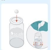
Add a DPD Nitrite tablet. Then, crush and stir.
