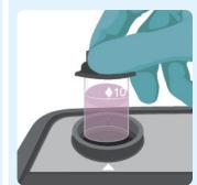
Place in the cell holder and press Measure. The Free Bromine result will be displayed. Press Finish to scroll through all the results in this test.
