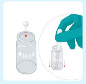
Add a DPD 1 tablet to those drops. Then, crush to form a paste.
