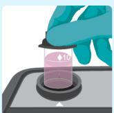
Place the tube in the cell holder and press Measure to obtain the concentration of Total Bromine.
