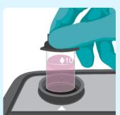
Place the tube in the cell holder and press Measure to obtain the concentration of Total Bromine.
