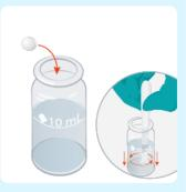
Prepare sample by adding a Calcicol No1 tablet. Crush and stir.
