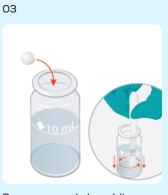
Prepare sample by adding a Calcicol No1 tablet. Crush and stir.
