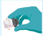
Remove any bubbles by holding tube horizontally and rotating.
