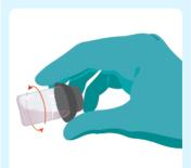
Remove any bubbles by holding tube horizontally and rotating.
