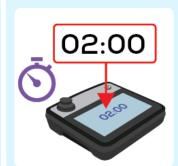
Allow timer to count down 2 minutes. The concentration of Total Chlorine will be displayed. Press Finish to scroll through all Chlorine results.
