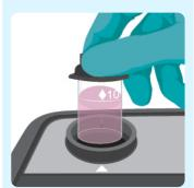
Place the prepared sample in the cell holder and press Measure to obtain the concentration of Free Chlorine.
