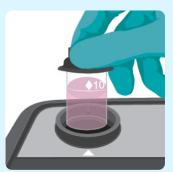
Place the tube in the cell holder and press Measure to obtain the concentration of Free Chlorine. Then, press Continue.
