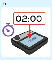
Allow timer to count down 2 minutes. The concentration of Total Chlorine will be displayed. Press Finish to scroll through all Chlorine results.
