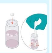
Continue, using the same sample. Add a DPD 3 tablet and crush and stir.
