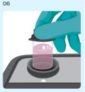
Place the prepared sample in the cell holder and press Measure to obtain the concentration of Free Chlorine.
