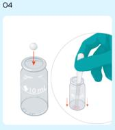
Add a DPD 1 tablet to those drops. Then, crush to form a paste.
