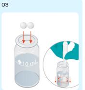
Prepare sample by adding an Acidifying GP tablet and a Chlorine HR tablet. Then, crush both tablets and stir.
