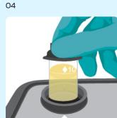
Place the tube in the cell holder and press Measure to obtain the concentration of Total Chlorine.
