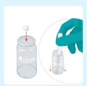
Add a DPD 4 tablet to those drops. Then, crush to form a paste.
