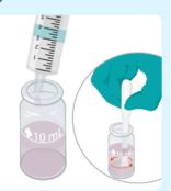
Fill to the 10 mL line with further sample and stir.
