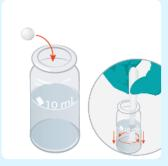
Prepare sample by adding a Fluoride No1 tablet and crush and stir.
