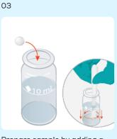
Prepare sample by adding a Manganese HR No1 tablet. Then, crush and stir.
