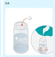
Then, add a Manganese HR No2 tablet. Crush and stir until fully dissolved.
