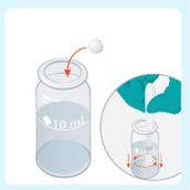
Then, add a Manganese No2 tablet and crush and stir.
