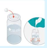
Prepare sample by adding a Manganese No1 tablet and crush and stir. Note: Sample temperature needs to be between 19°C and 21°C.
