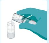
Carefully decant 10 mL of clear liquid in to a photometer tube.
