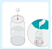
Then, add a Nitricol tablet and crush and stir.
