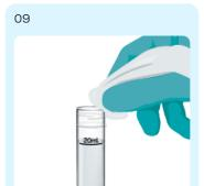
Remove cap and wipe rim to remove all traces of Nitratest powder.
